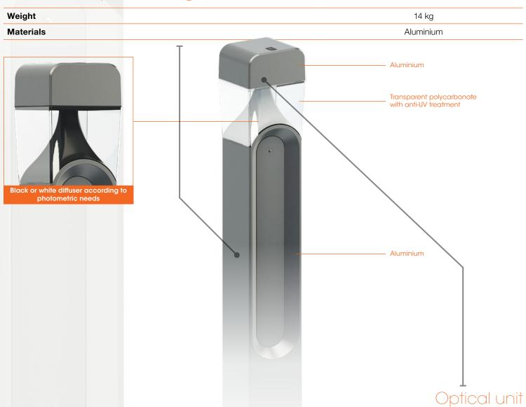
8 or 16 LED PCB - From 980 to 3800 lm (see attached AIR datasheet for details on power, light intensity and photometry available). Integrated smart driver (control, automatic adjustment, CLO, graduation via voltage variation or DALI). ULR < 1% (ULR: Upward Light Ratio).
